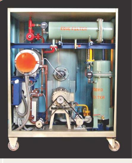
What is the essential to filter the Quenching oil? As metal is quenched in an oil shower, fines frame in the Quenching oil from the cooling procedure. Particles including carbon particles and little bits of blaze are added to the Quenching oil after some time. As these fines develop in the encompassing quench fluid, they can influence the quench in any number of ways.
